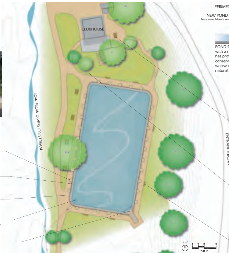
The existing asphalt surface of the pond has proven over time to not be the appropriate material to contain the pond water. It is old and has been deteriorated over time.
